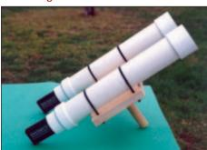
■ FIGURE 8. Pair of "Sonic Super Ears" used for the microphone/amplifier systems. The plastic case of one of the microphone/amplifier systems is shown cemented into a 2 x 1-1/2 inch PVC pipe increaser using Gorilla Glue.
