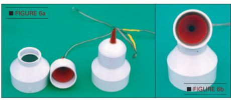
■ FIGURE 6. Close-up views of the funnel/microphone/end cap assemblies. (a) Left end-cap unassembled; right end-cap in final configuration. (b) Close-up of funnel in end-cap; the electret element has been glued into place about 1/2 inch down the exit throat of the funnel stem.
