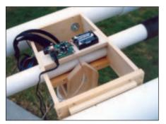
■ FIGURE 4. Placement of the battery holder for three AA batteries and of the Velleman "Super Stereo Ear" printed circuit board is visible, along with a close-up look at the altazimuth mount construction.
