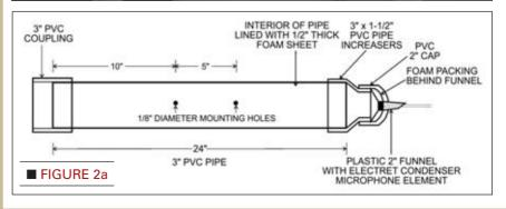
■ FIGURE 2. Construction details and dimensions for the microphone tubes and mount: (a) Microphone tube; (b) Interior section of the altazimuth mount; and (c) Front of altazimuth mount.
